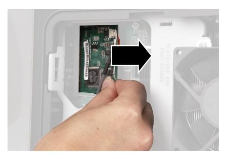
**5** Remove the cable from the Mini-PCI card.
